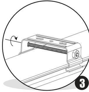
Insert Tensioning Bolt and attach the Batten Light to the metal clips.
