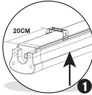
Fix the two metal clips into position and attach to surface. It is recommended that each clip is positioned approximately 20CM from each end of the Batten Light. Caution : Ensure correct anchor sleeves are used for surface material. Please see package contents before installation.
